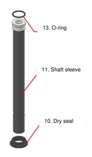
5) Pull the shaft sleeve (11) up from the shaft and remove it. At that time, remove the dry seal (10) and O-ring (13).
