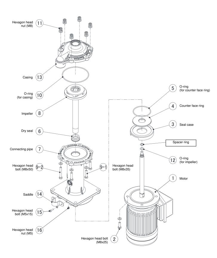
■ Note 1: Cautions on loosening/tightening the impeller.
