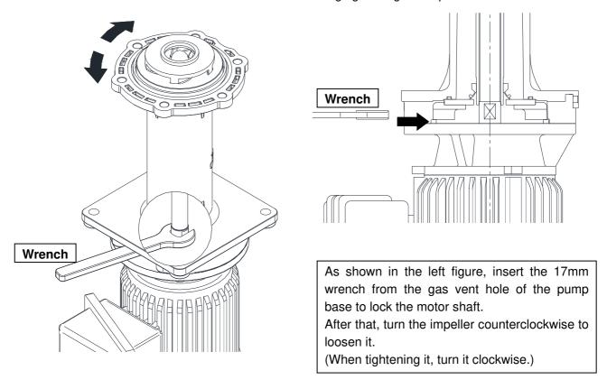
■ Note 2: Seal case/pump base installation.
