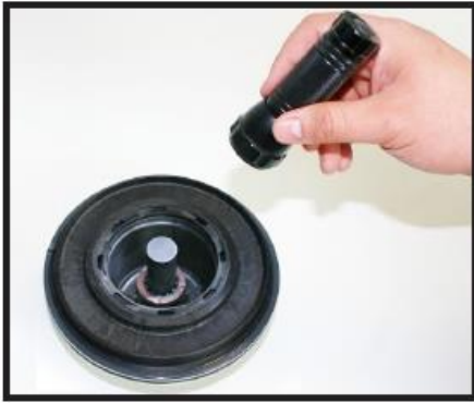
Use a flashlight to check the inside of the rear casing.
