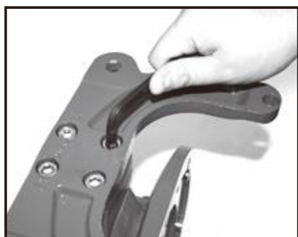
Tighten 4 cap screw by using a hex. wrench.
