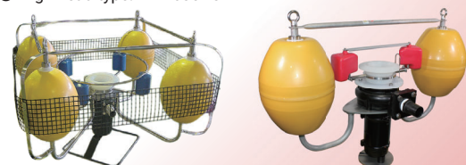
Double-float structure (YouTube) 1500PS Crushing type Aquatic weed collection (YouTube)
